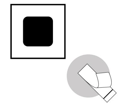
1 Separate the silver disc with the adhesive strip from the black magnet. Remove the protective film from the adhesive strip.
