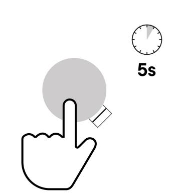
2 Use the adhesive strip to attach the disc onto the wall and press down for at least five seconds.
