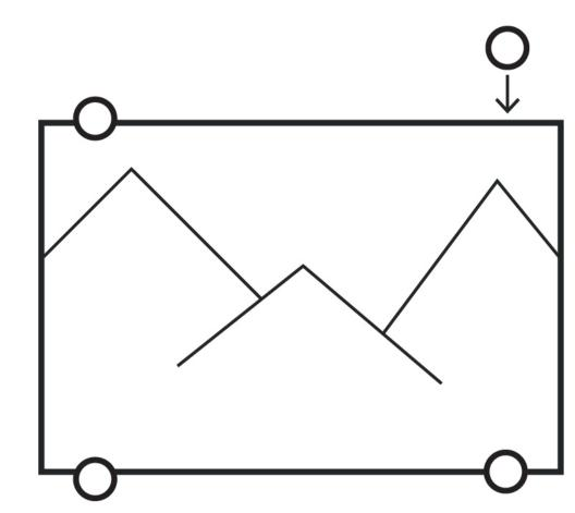
Place the plate holders on the upper and lower edges at the required distance from the corners (for example 5 cm).
