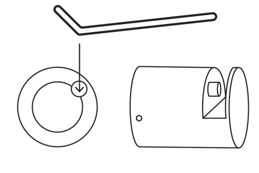
2 Tighten the four plastic screws from behind with the Allen key until there is a noticeable increase in resistance. Measure the distances between the centres of the large mounting holes in the plate holders and transfer the positions to the wall.
