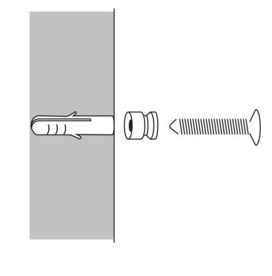
**3** Use a 6 mm drill and press the dowel plugs fully into the wall. Push the screws into the fixing sleeves and screw them into the dowel plugs.
